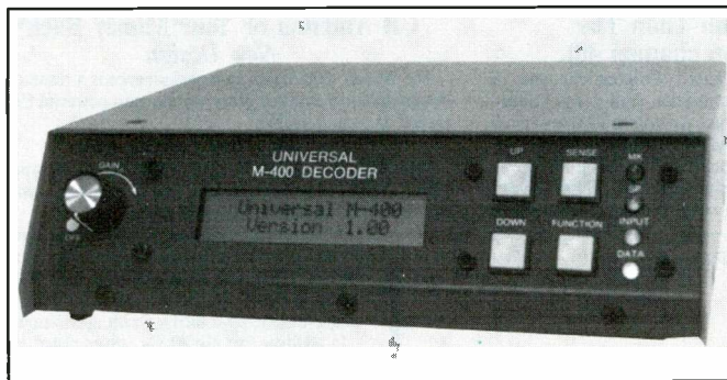
Universal's M-400, used on both VHF/UHF bands, decodes aircraft traffic, pagers, and CTC/DCS signals.
