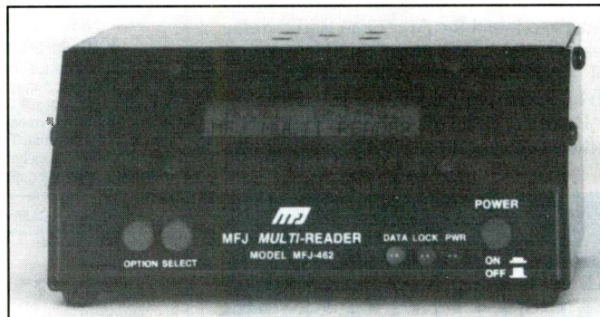
The MFJ-462 Multi-reader continuously offers solid copy even with signals buried in noise. A precision tuning indicator aids in adjusting the receiver.
