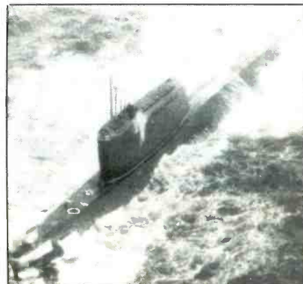
HOTEL II-Class SSBNs carry three SLBMs and eight torpedoes. They are in radio contact with surface vessels.
