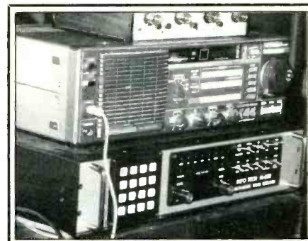
At the bottom of this stack of gear is an Info-Tech M-600 multi-mode RTTY decoder, one of the more sophisticated units available to the monitoring enthusiast. It's capable of unraveling RTTY/ARQ/FEC and even CW. It also cracks "bit inversion" privacy codes!
