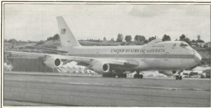
The USAF AABNCP can fly for up to 72 hours during a national emergency. It has VLF communications facilities.
