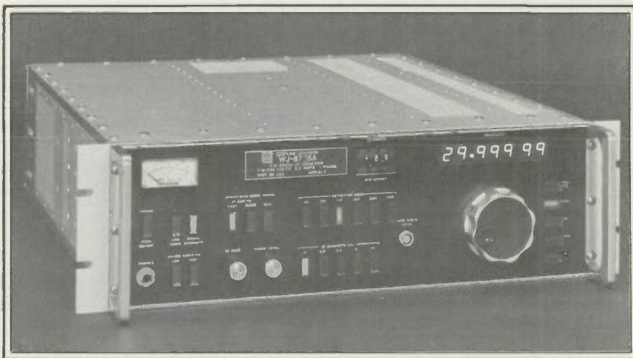
A very sophisticated, modern receiver covering these frequencies is the Watkins-Johnson Company's WJ-8718A. It covers 5 kHz to 30 MHz in all modes.
