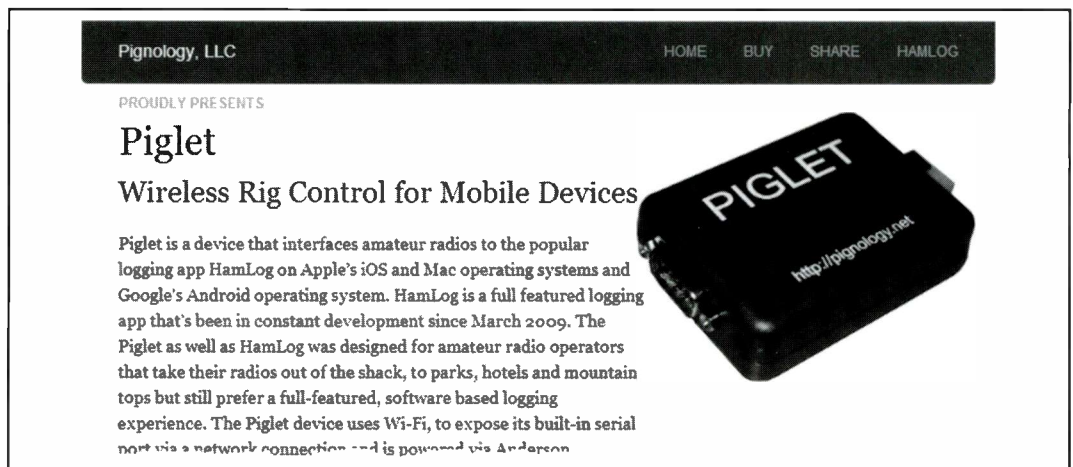
Photo A. The Piglet pigtail device provides a way to remotely control a rig from an iPhone, iPad, or Android device. (Internet screen grab < http://pignology.net/piglet/ >)
