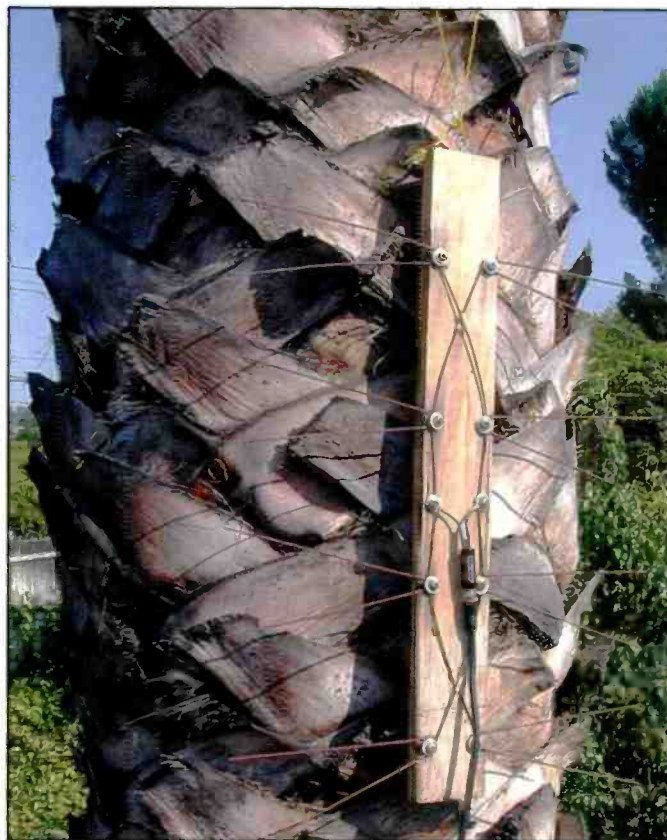
Photo A: This little homebrew DTV antenna's coat-hanger elements have turned rusty red, which helps it blend nicely into the side of a palm tree — and is barely visible from the ground. (Courtesy of K16SN)
