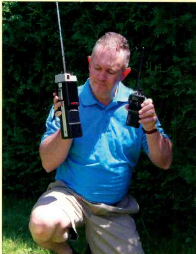
The CB handheld radios of today — such as the Midland 75-822 — are tiny compared to Radio Shack's Realistic TRC-209, circa 1970s — a large, three-channel, vintage 2-watt transceiver fashioned after the large handie-talkies used in World War II. The '209 is one of the favorites in Jeffrey Reed's collection of portable CB radios. (Courtesy of Jeffrey Reed)
