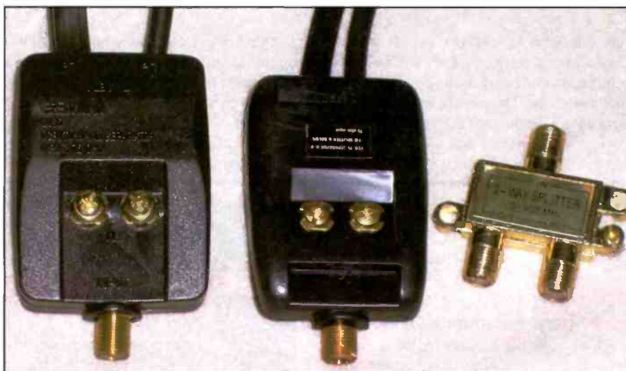
Photo E. FM band splitters to take the FM signal off an outdoor TV antenna.
