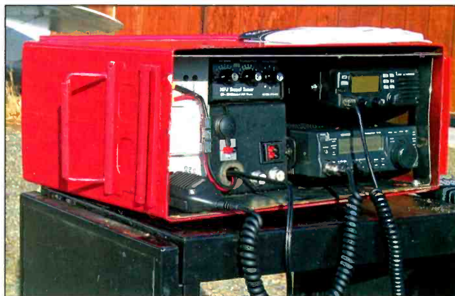
These are "before" and "after" shots of Frank, KLØSW's Bug-Out-Box (BOB). Frank's BOB features a large rechargeable (sealed lead-acid) gelled-electrolyte 20 A/hr batter which is recharged by the A&A Electronics "smart charger." The VHF unit sits above the HF transceiver in the BOB. Deployment is pretty straightforward and Frank can be on the air quickly once he arrives on station.
