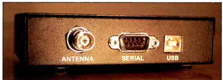
The SDR-IQ rear panel with antenna, serial, and USB connectors.
