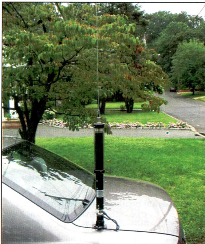
Here's the Little Tarheel II mounted on the trunk deck of our vehicle using the MFJ-348T. The antenna not only looks good, it's a great performer and ideal for mobile SWLing/DXing and even CB!
