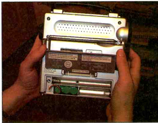
Sometimes you need a crowbar to open a radio battery compartment, but accessing the FR300's battery compartment is a simple two-finger operation!
