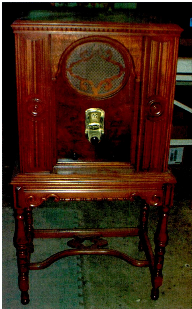
Photo A. I took this photo of the restored Majestic when the chassis, speaker, and power supply sections were reunited with the refinished cabinet at the furniture restoration shop.
