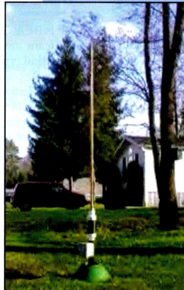
Nice Sticks! The www.sstran.com site shows construction details for a high-efficiency Part 15 compliant AM antenna system with loading coil and transmitter mounted at the base ( www.sstran.com )
