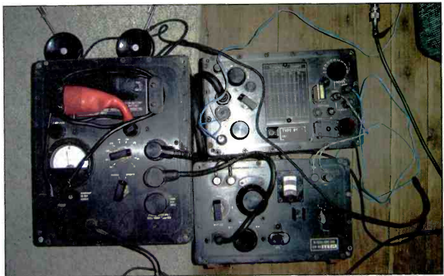
Shown here is the venerable GRC-109 "spy set" used by the CIA and the U.S. Special Forces (Green Berets) from the 1950s into the 1980s. The three boxes shown here comprise the basic radio set. This set can be powered from various sources of AC, 6 VDC, and a hand-cranked generator. The complete radio set weighs in at over 50 pounds and would be a real treat to jump with into a hostile drop zone.
