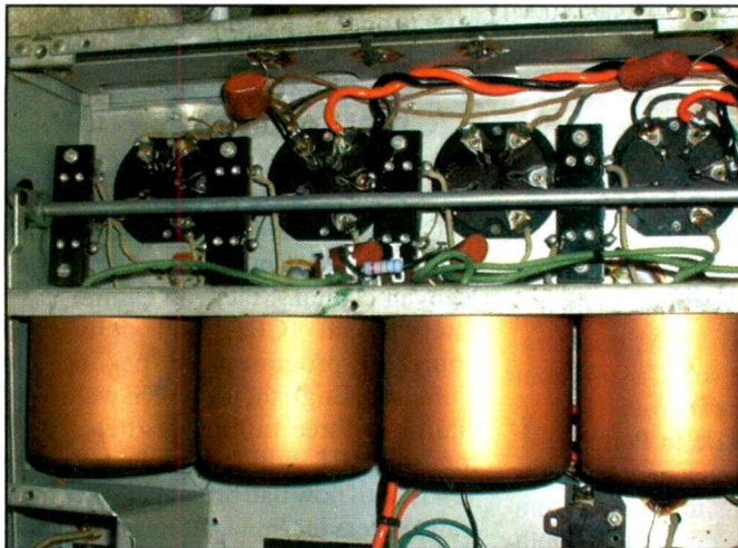
Photo E. A close-up view shows the TRF RF stages and coil assemblies.
