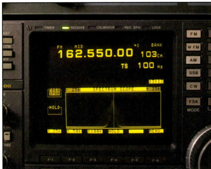
Here's a signal that's right on frequency. You can see the bandwidth represented on the spectrum scope by the width of the signal centered on the vertical line.
