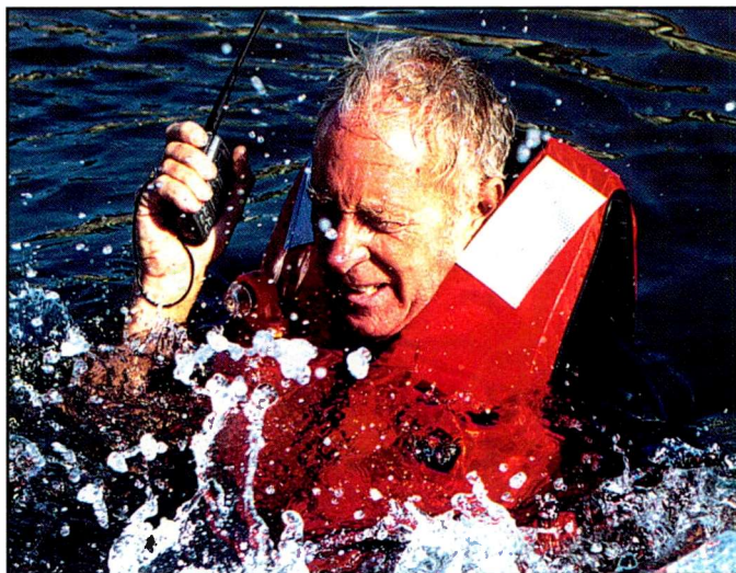
Each radio was turned on and held under water for two minutes.
