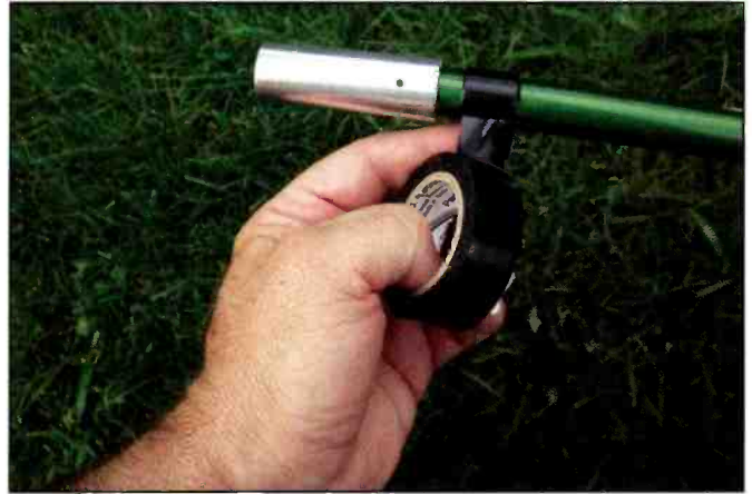
All fiberglass pole joints are securely taped with the provided electrical tape, then covered with a special self-sealing tape. This photo shows the tip of the antenna being prepared for the vent cap.
