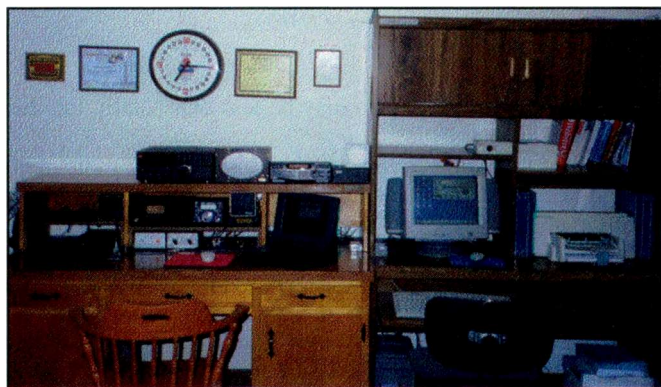
Here we see Charles' very well organized computer-assisted monitoring station. On the left are his three main radios on the top shelf of the desk. From left to right are the Japan Radio NRD 535D, Uniden BC895XLT and the Ten-Tec RX-320. The computer control is accomplished by the laptop on the desk and the tower style computer in the computer hutch to the right (note the radio control programs that are displayed on both computer's video screens).
