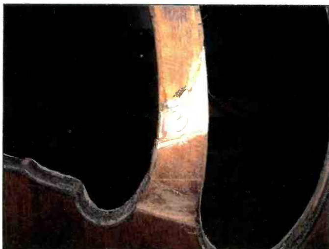
Photo J. Tiny pieces are fitted where gaps remain between salvaged original pieces. Here, the patch lies over one of the speaker mounting holes.
