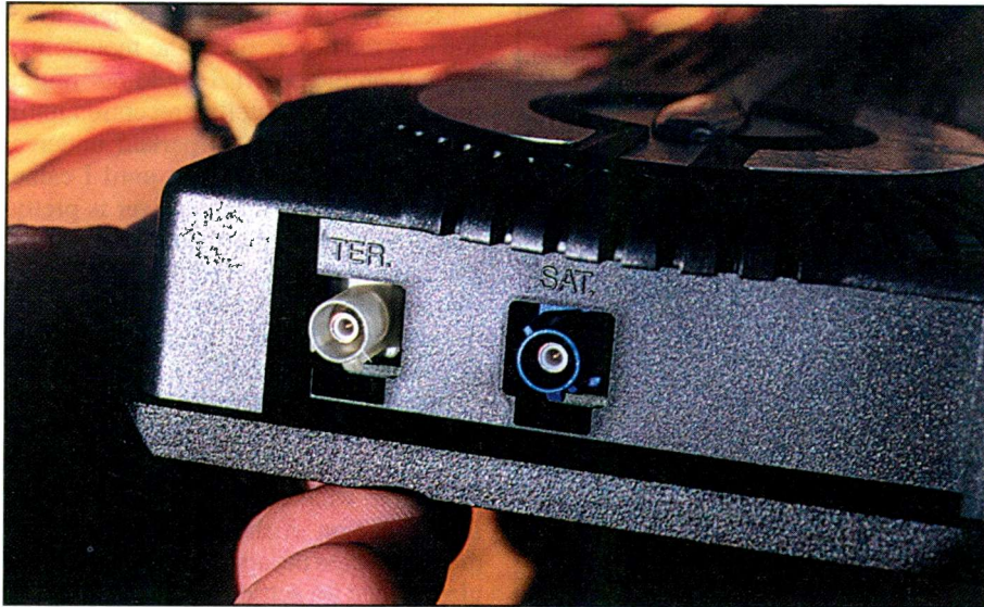
The Shakespeare antenna gives two inputs—terrestrial for tuners, and satellite direct.
