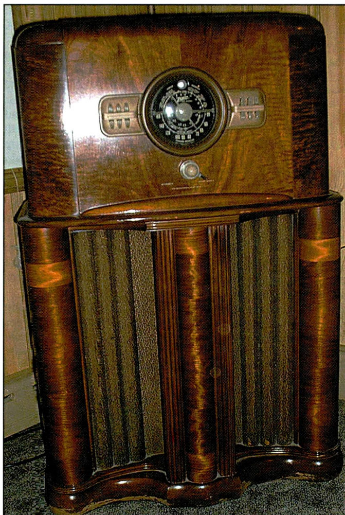
Photo A. The author's Zenith 11S474 console. The radio was found at an estate sale and is in exceptional condition. This 11-tube console is a real bandcruiser on AM and sounds as sweet as it looks.
