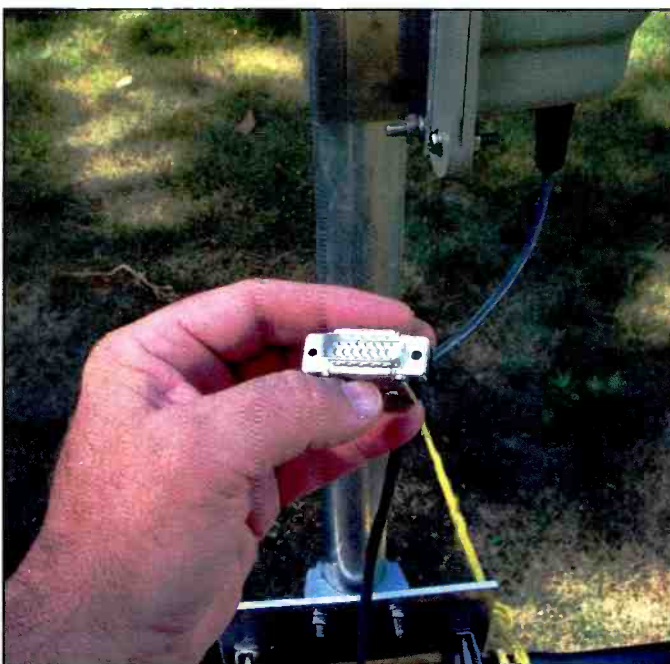
The 15-pin male connector gets filled with silicone grease (included), then plugs into the included wiring harness, which then plugs into the antenna.
