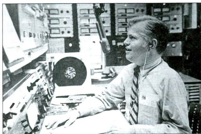
A rare glimpse at CBN Northeast master control operation in Ithaca, New York, circa 1972. Andrew "Andy" Anderson is on the air. Through the CBN Ithaca-based FM transmitter/antennas there, Anderson's voice is being broadcast to a series of four other Empire State transmitter sites capable of covering media markets from Albany to Buffalo. Especially interesting in this photo is the row of modulation monitors and remote control units (in background) that allowed CBN to "read the meters" and check each transmitter's audio without having anyone at the Wethersfield, South Bristol, DeRuyter, or Cherry Valley sites. That technology saved salaries that the stations' founders (Rural Radio Foundation) had once paid out to a 19-member engineering staff!
