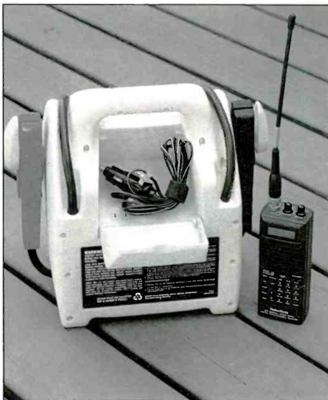
The rear of the Jump It! has a handy compartment that holds the included AC adapter with ample room for your small 12 Vdc radio-to-battery cord.
